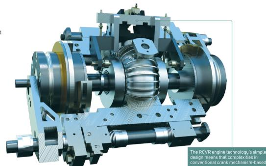
downsizing gains inherent with VCR by means of its two double-acting pistons producing power at every stroke while cutting down on FHP and piston chattering losses.
